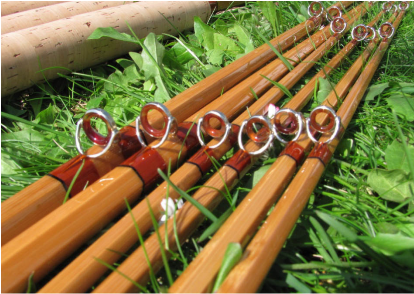
The finished rods, 12'6" and 13'0", with agate-guides throughout. A total of 57 guides plus 6 agate tip-tops.
