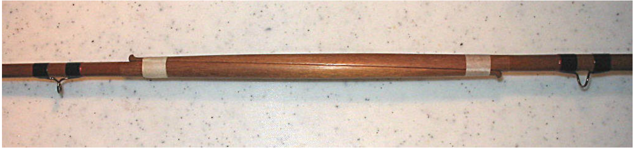
Playfair Grant Vibration 13 foot rod. Butt splice. Note the dramatic swell over the splice.
