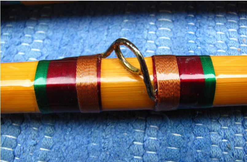
Details from above rod, note the copper-wire over silk at the guides and female ferrules.
