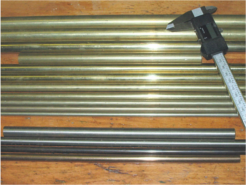
Solid stock top Ni-Si, bottom Titanium and Al-Bronze
