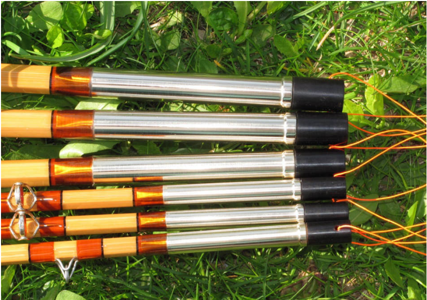
Females installed, with ebony-stoppers
