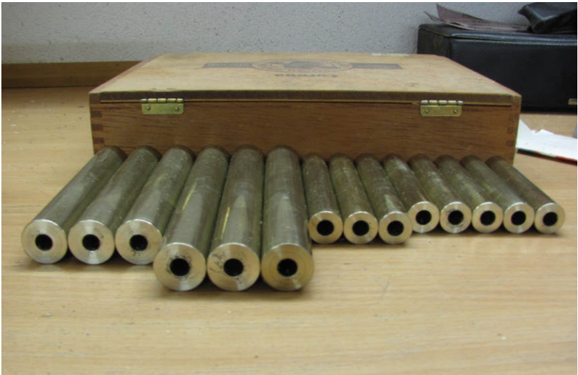
Initial holes drilled through. I use a hard metal drill for the pilot-hole
