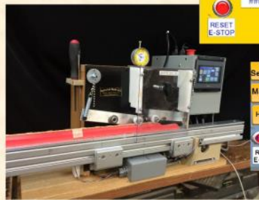
The new Programmable Cane Mill Finished strips in 2 passes. Touch screen control. Click to watch the video
