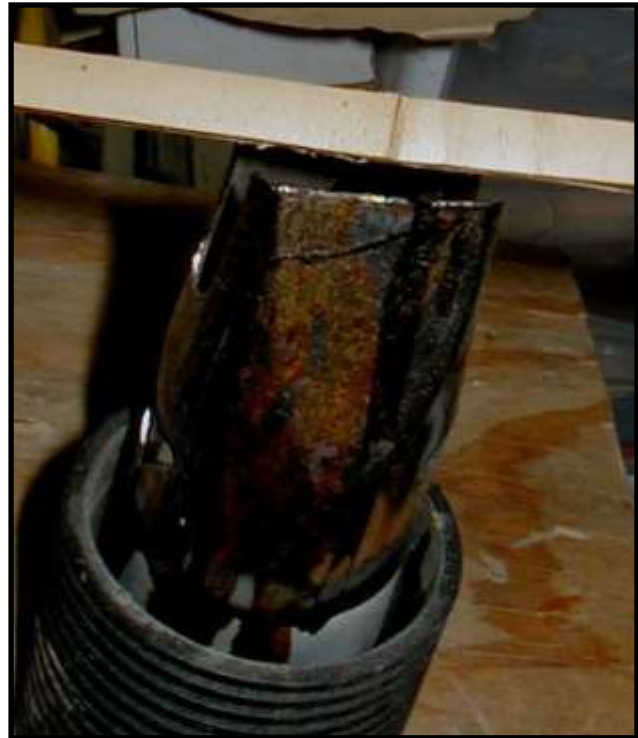
Heating the soaked node. It takes less than a minute to heat the node. No burning or hardening on the nodal area.
