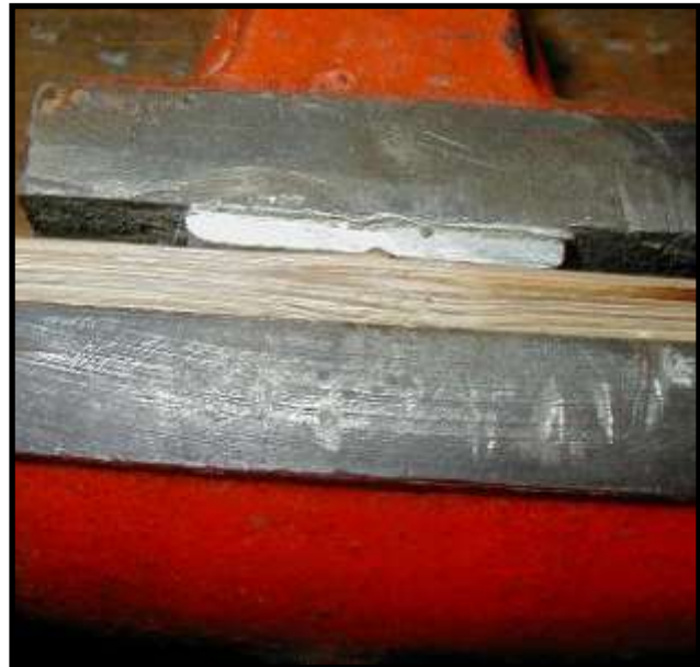
The node is now displaced into the recess previously sanded. Note there is a groove in the plate to accommodate the ridge.
