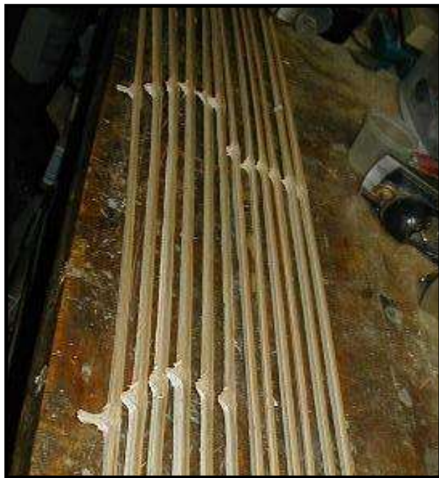
Staggered nodes, note the dams.
