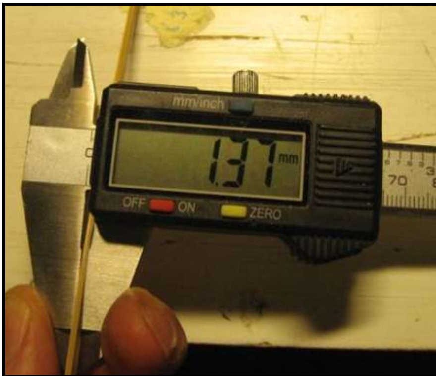
Thickness of the strip is here 1.37 mm (= 0.054").
