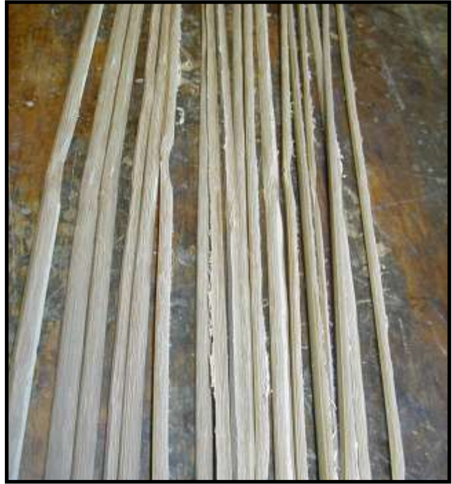
Recessed and rough 60 sanded.
