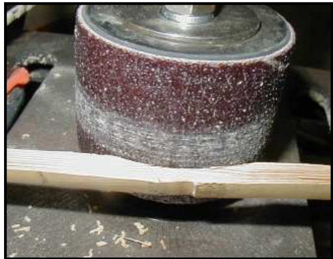
Inner dam sanded recess sanded, this recess is to accept the depressed node.
