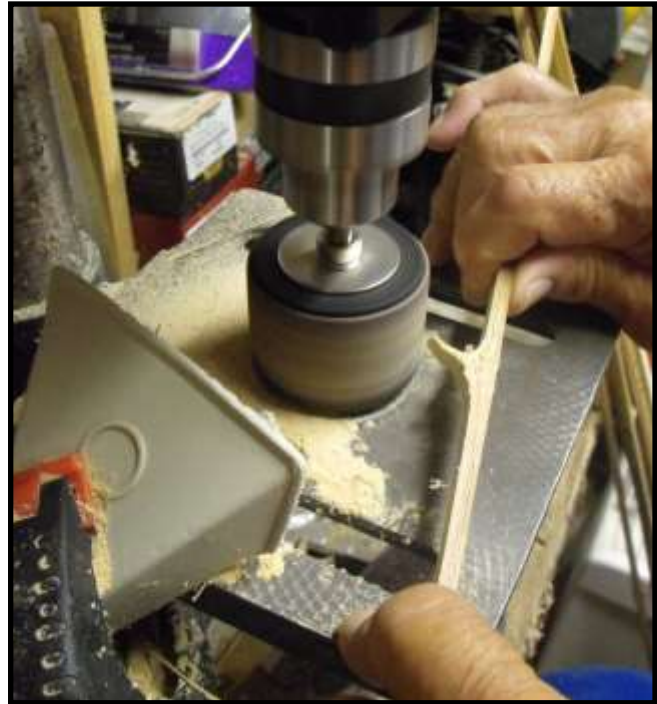
Removing the inner dam.
