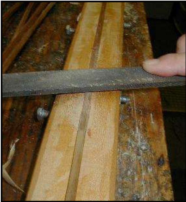
The node ridge is removed with just a few passes of the file. The bump is displaced so not much of it will be filed. This keeps more power fibers from being removed from the bump.
