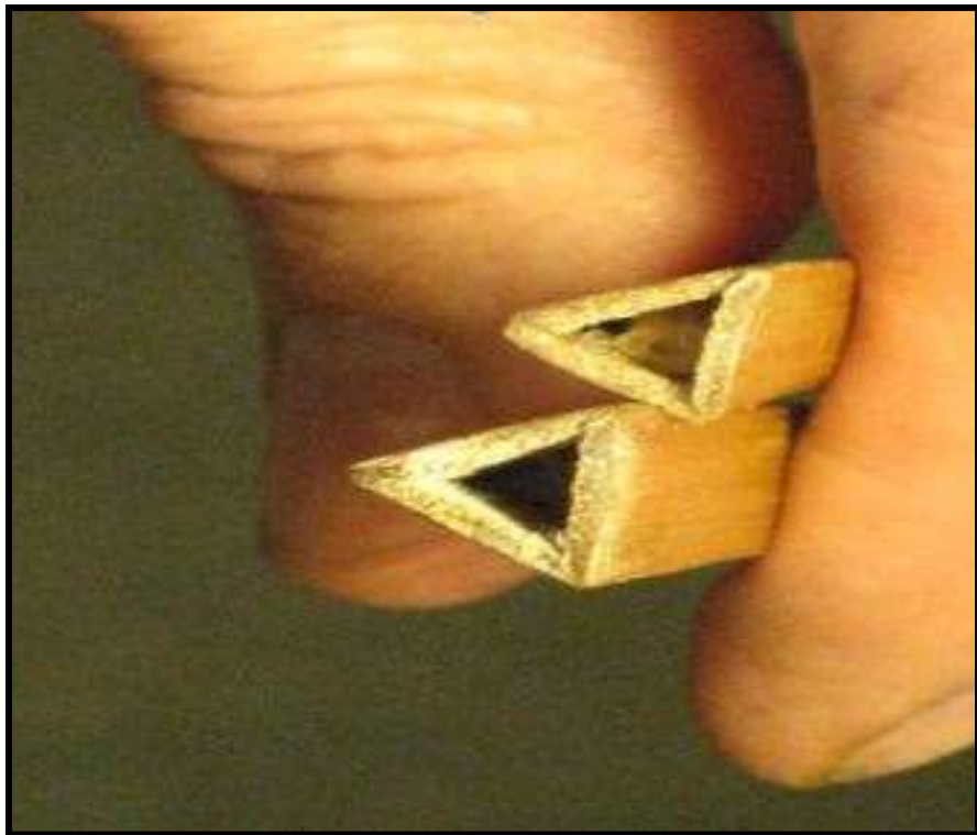
Triangle hollow-built rod cross section.
